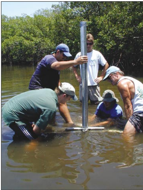
Retrieving a sediment core from Tampa Bay.
