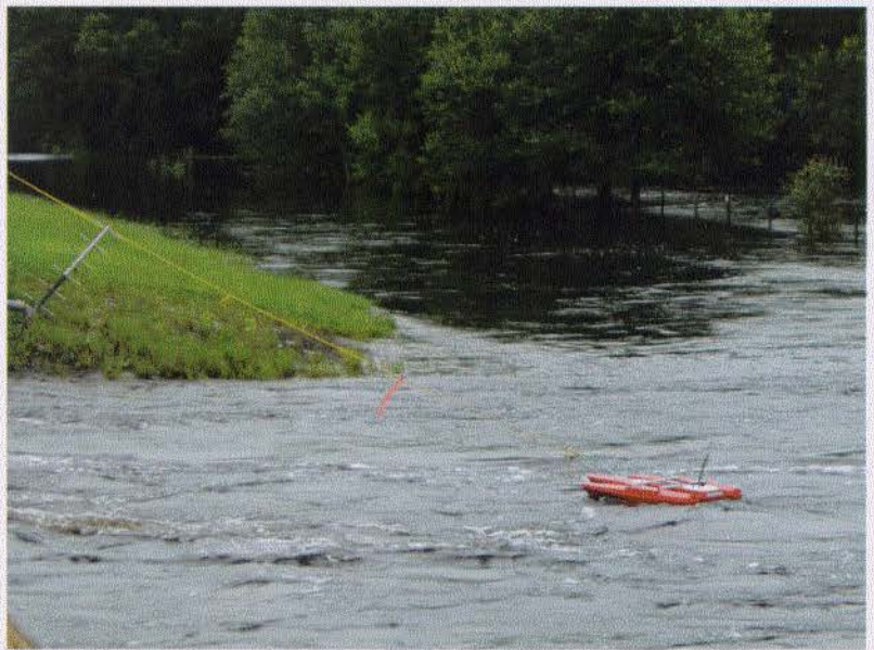
Figure 4 —View of Big Slough Canal near Myakka City (site 7, fig. 1, table 1). Discharge measurement being made using a tethered boat and acoustic doppler current profiler.
