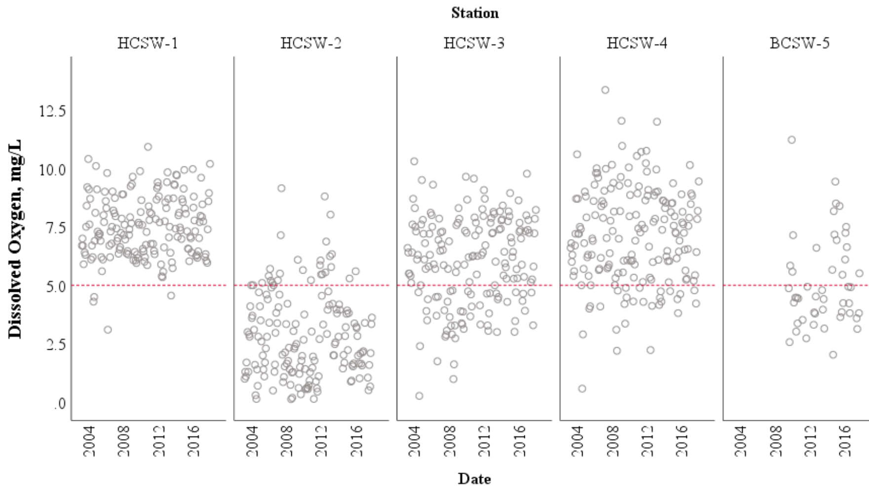
Figure C-2 Dissolved Oxygen Concentrations Obtained During Monthly HCSP Water Quality Sampling Events, 2003-2018. This analyte was discontinued in 2018.
